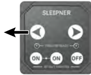
Activating both bow and stern thruster to rotate the boat on axis
