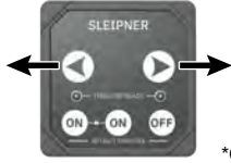
Activating the bow thruster
