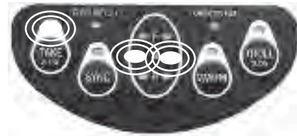
TAKE light and gear indicator lights flash at station that is INACTIVE
