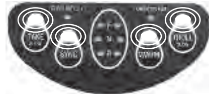
All 4 lights flashing in unison indicates system is in ALARM Mode
