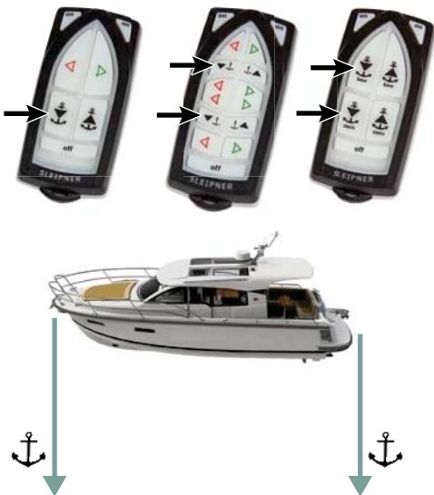
Activating lowers Anchor/Windlass
