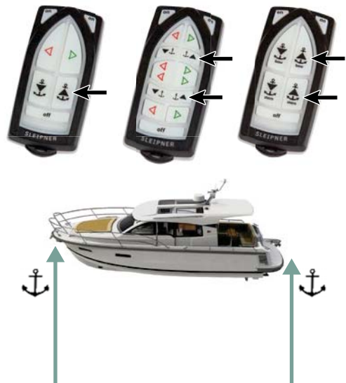
Activating raises Anchor/Windlass
