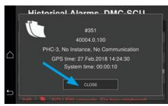
If an alarm occurs so the stabilizer system is not running, but the fins are centred and locked, you can operate the boat normally, remembering the general warning about high speeds and inactive stabilizers. See Alarm list and boat handling restrictions in table below for more details.
