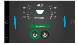
Note! System change automatically between Cruising/ At Anchor when both is activated.
